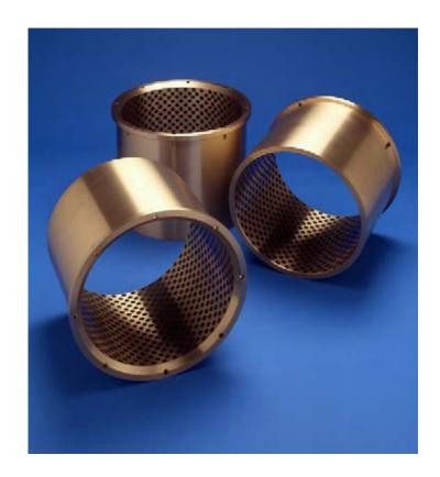
LUBRON AQ30 lubricants are embedded into circular recesses provided for containment of the lubricant. Covering 30% to 40% of the bearing surface, these recesses securely anchor the lubricant and provide permanent reservoirs for restoring the bearing surface.
